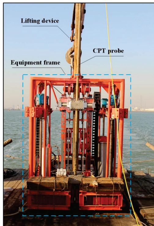
Figure 2. Underwater CPT system, developed independently.
