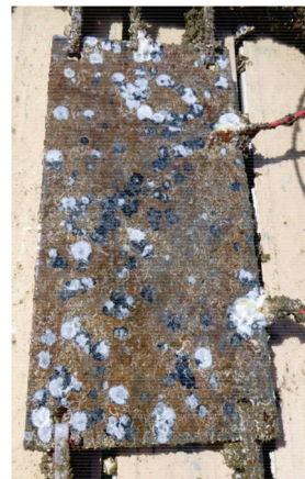
Figure 10. Condition of the initially clean panel after scraped off.
