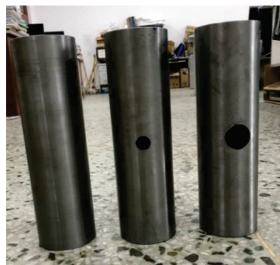
Figure 15. Steel tubes with three different damage holes.
