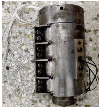
Figure 16. Fully assembled clamp for experiments.
