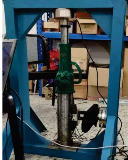
Figure 18. Axial loading of the steel pipe.
