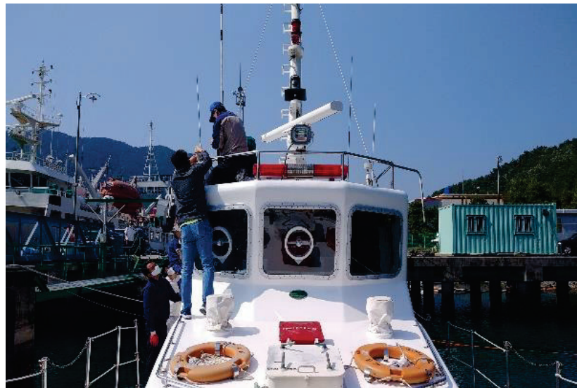
Figure 1. Automatic Identification System (AIS) and V-pass antennas installed at the same place on the ship.
