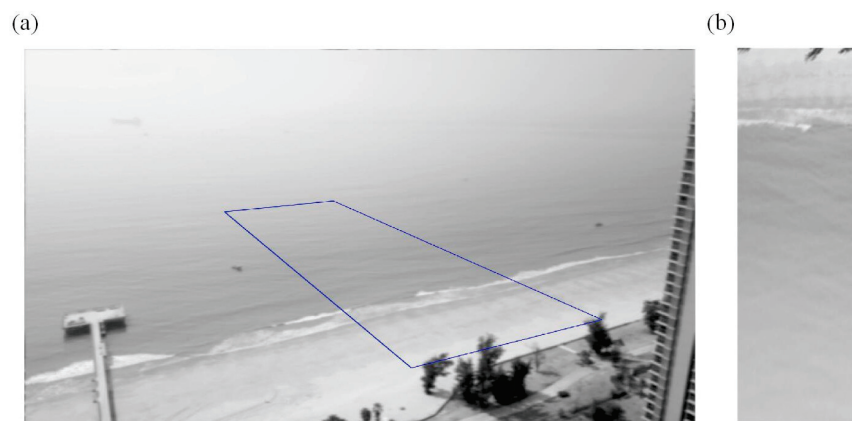
Figure 8. Schematic diagram of interest region selection. (a) The target area is shown in the blue line in the original scene image. (b) Unified pixel resolution orthoimage.
