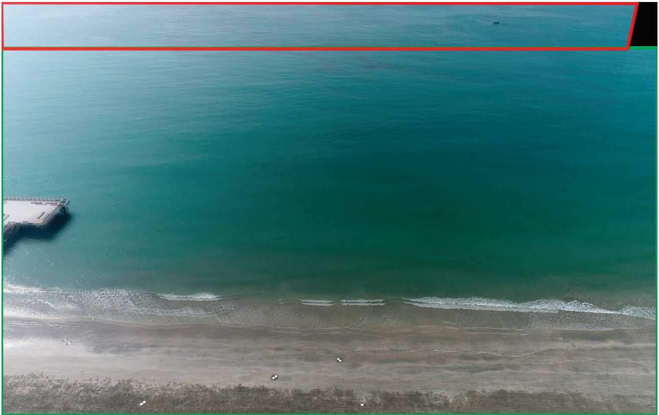
Figure 27. The green rectangle is the FOV of a single UAV. The red is the extension of the stitching.
