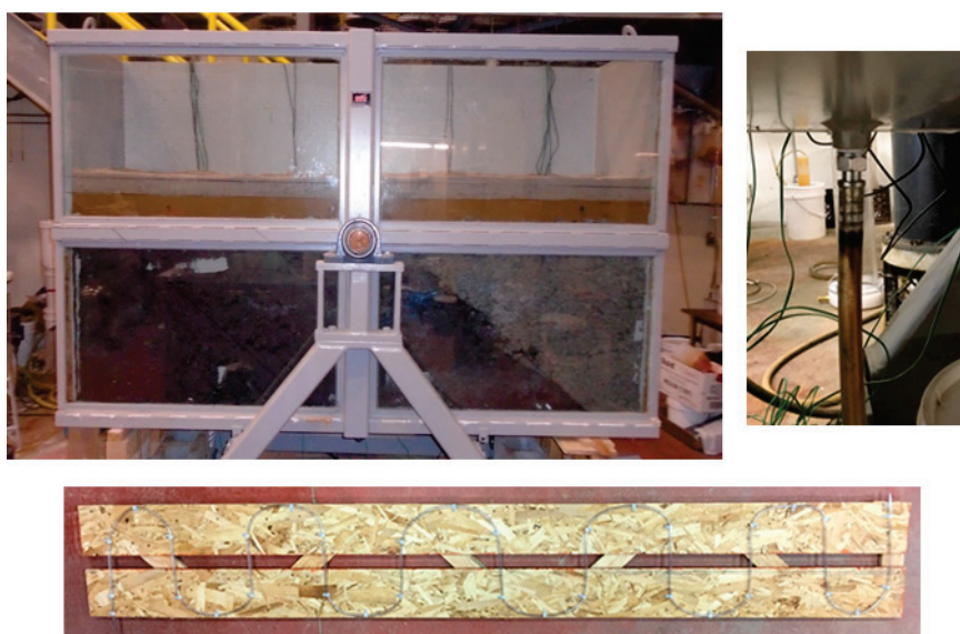
Figure A1. Photos of the laboratory experimental set-up. Top left: Front view of the laboratory scale model. HI rock is the dark grey material on the left which was deposited in three segregated zones; anorthosite is the light grey material (to the right of the HI); sand is orange-brown in colour along the top with crushed anorthosite (light grey) above to form the FCL. The tank was pivoted at an angle of 5° for the duration of the experiments with steady-state flow rates. Top right: Drainage tubes 1 cm in diameter that allow effluent to freely drain into the collection buckets below. Bottom: Set up of tubing with drainage holes installed along the top of the lab model to distribute the water applied at 180 L day -1 .
