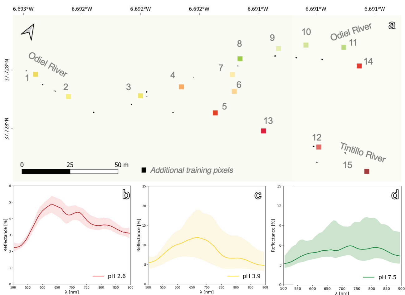
Figure 6. (a) Created training dataset based on 15 ground-truth georeferenced stations. Mean spectrum of the clustered pixels used in the training dataset and standard deviation plotted as shaded envelope. (b) pH 2.6 ( \sigma = 0.16 ), (c) pH 3.9 ( \sigma = 2.01 ), and (d) pH 7.5 ( \sigma = 0.98 ).
