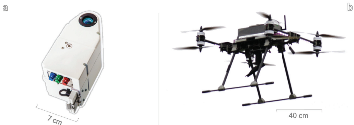
Figure 3. Overview of the unmanned aerial system (UAS) used for image acquisition: (a) The Rikola hyperspectral (HS) camera [24] mounted on the (b) Tholeg UAS.
