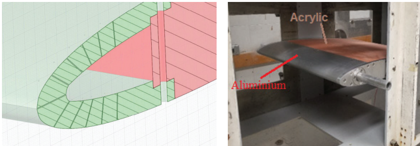
Figure 5. Two different materials of the model: aluminium alloy (hollowed out) and acrylic.
