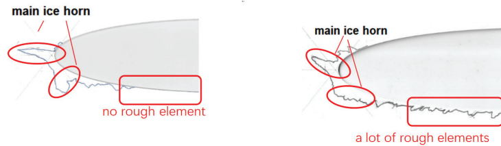
Figure 14. Ice shape of normal drop (left) and SLD (right).
