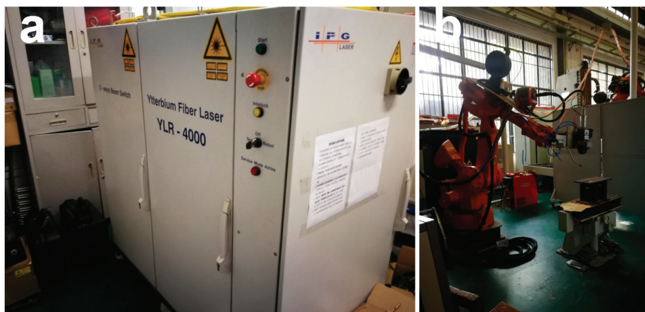
Figure 5. Welding devices: (a) IPG YLR-4000 fiber laser; (b) ABB IRB4400 robot.
