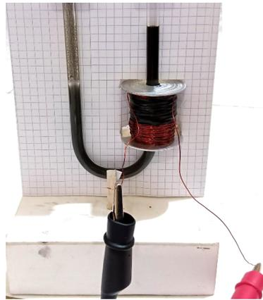
Figure 1. Different MRFs levels in both legs indicating a pressure change.
