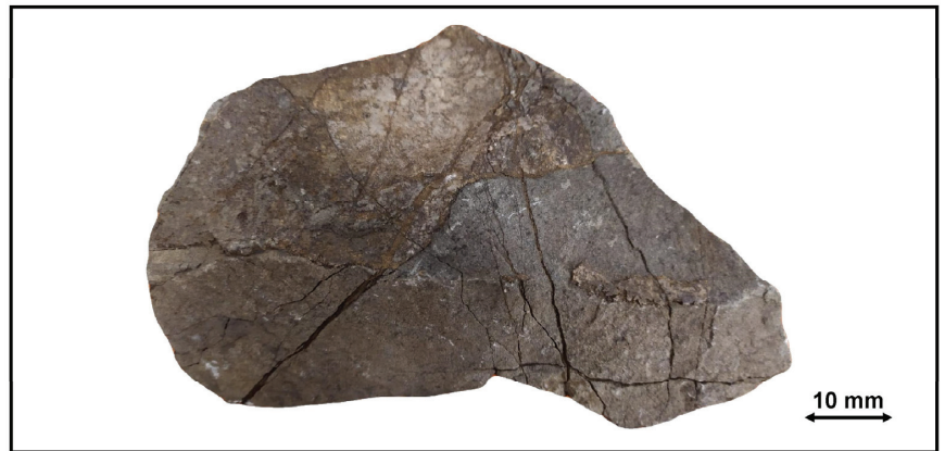
Figure 1. Sample of waste dump showing cracks filled with hydrothermal chemical compounds.
