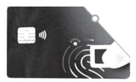
Figure 2. NFC banking card sample equipped with a fingerprint.
