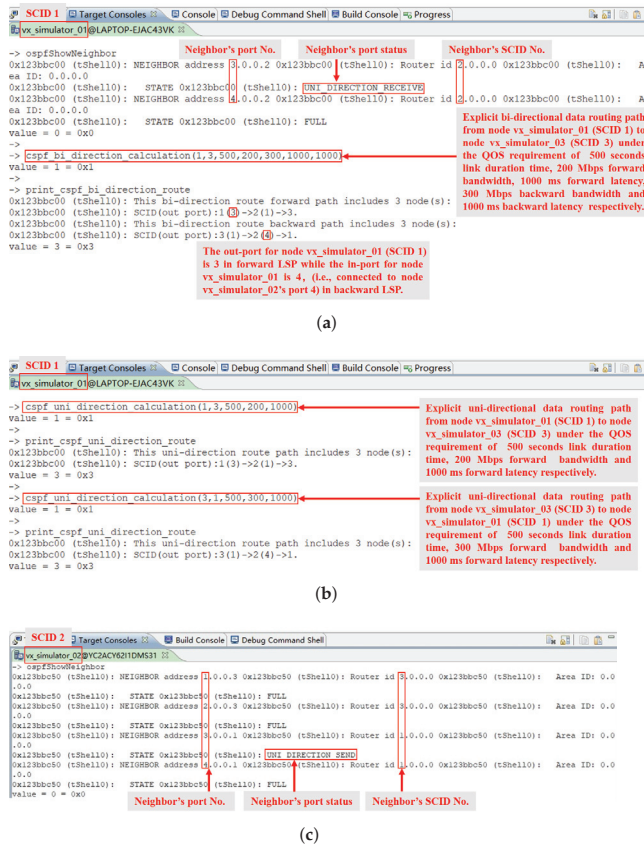
Figure 24. The explicit constraint data routing computation under QoS requirements and the circumstances of uni-directional link between node vx_simulator_01 (ingress LER, SCID 1, uni-directional sending), node vx_simulator_02 (LSR, SCID 2, uni-directional receiving), and node vx_simulator_03 (egress LER, SCID 3). (a) The status of a neighbor's port and data routing computation in node vx_simulator_01. (b) The explicit uni-directional data routing path computation between node vx_simulator_01 and node vx_simulator_03. (c) The status of a neighbor's port in node vx_simulator_02.
