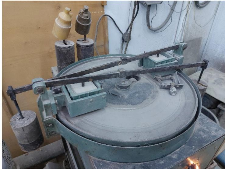
**Figure 6.** Abrasion resistance test. Composition samples No. 5 on a wheel tester.
