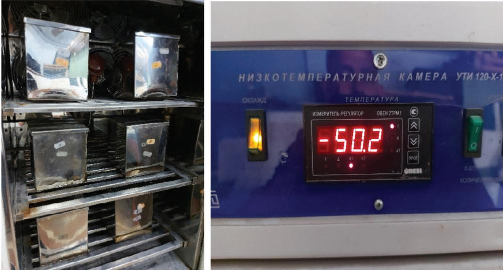
**Figure 7.** Frost resistance test.
