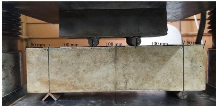
**Figure 2.** Flexural strength test using a 4-point load scheme.
