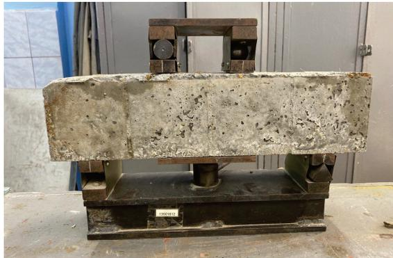
**Figure 7.** Four-point bend test setup.
