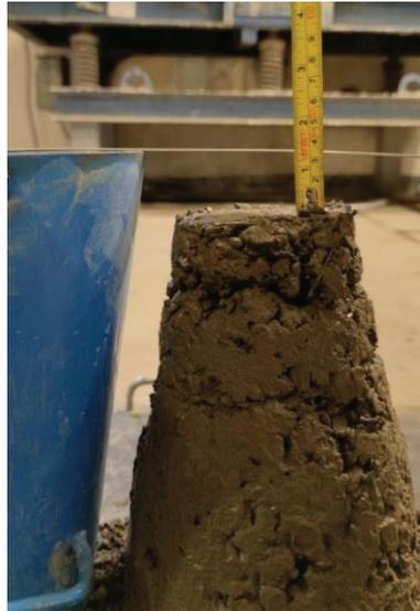
**Figure 1.** Slump test of the  $M_3$  concrete mix.
