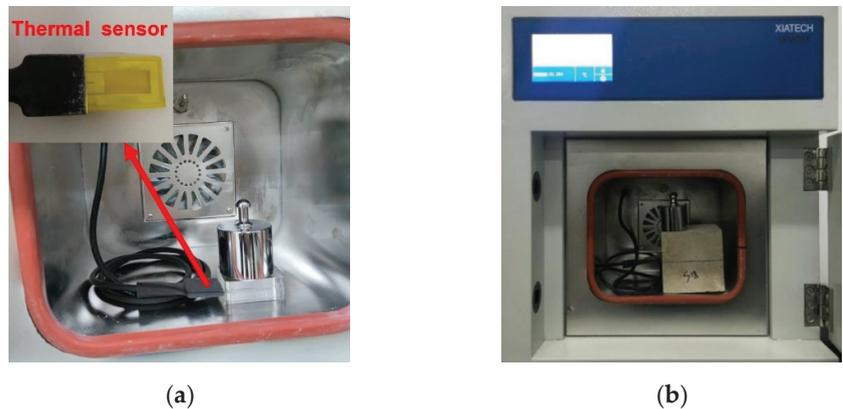
**Figure 4.** (a) Automatic test instrument for measuring thermal conductivity with hot wire method; (b) Thermal conductivity test of NAAC.
