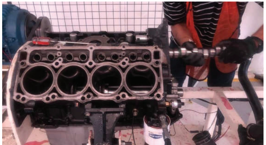
Figure 12. Removing the camshaft after complying with the test protocol.
