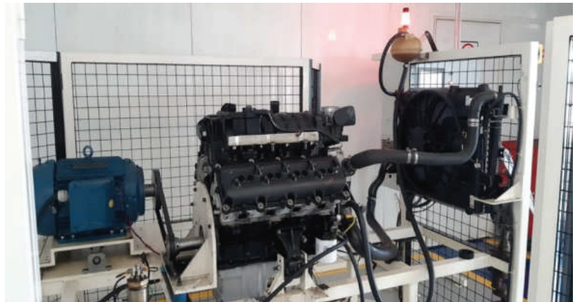
Figure 4. Electric Spin Rig machine—V8 engine 5.7L.
