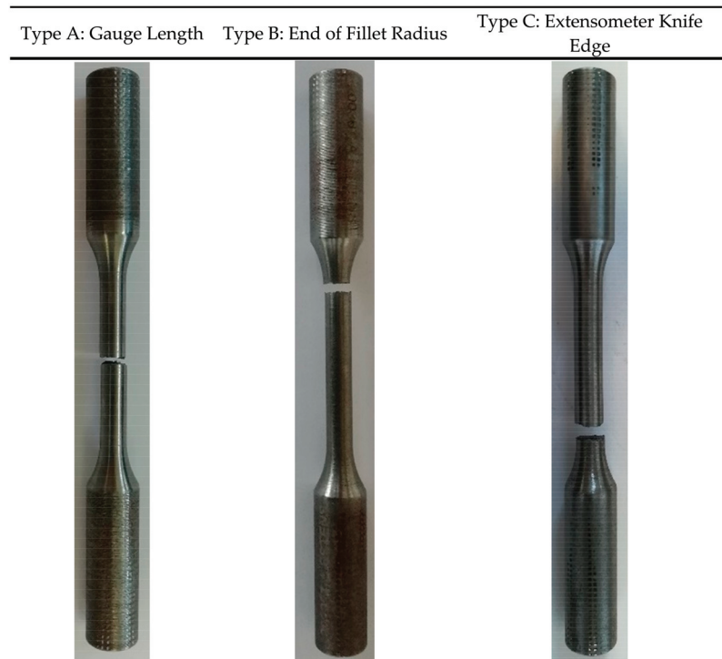
Figure 12. Failure locations observed after the static and the strain-controlled fatigue tests. The figure reports examples relevant to plain cylindrical specimens (Figures 4 and 5); however, the same definitions also apply to plain flat specimens (Figure 6).
