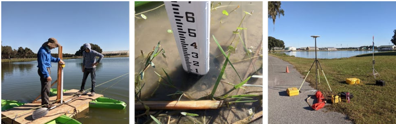
Figure 5. The moving rover and the data collector taking topographic points throughout the pond from a barge (left image). Custom 3D printed silt foot for level rod (center). The base station set up on a nail driven into the asphalt (left tripod) and the radio (right tripod) (right image) transmitting the RTK GPS corrections. The base nail was measured for 8 h as static observations and submitted to NOAA OPUS. Topographic points collected across different days were translated so that the base station points aligned with the NOAA OPUS solution. Photo credit: UF UASRP; student researchers pictured on the left image.
