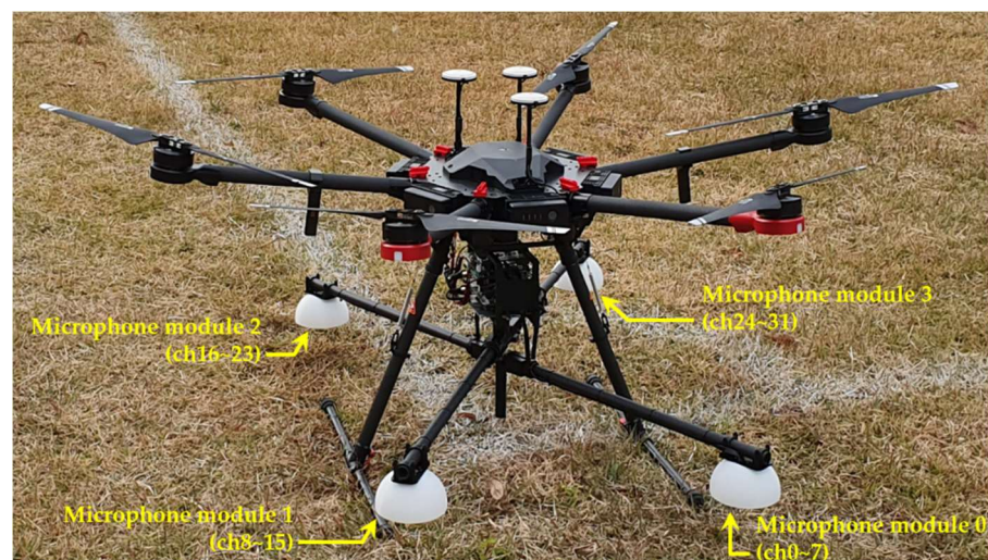
Figure 6. Microphone array system mounted on the drone.
