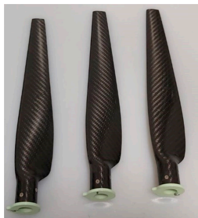
Figure 11. A Photo of the Rotor Blades Used for the Experimental Icing Tests.
