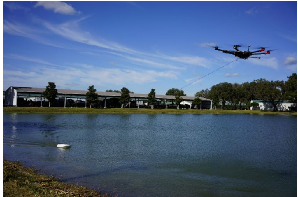
Figure 1. Bathymetry system during autonomous flight for ground-truthing at University of Florida Plant Science Research Citra, Florida. Photo credit: author's UF UASRP lab.
