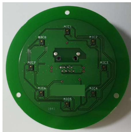
Figure 5. Microphone module consisting of 8 microphones.
