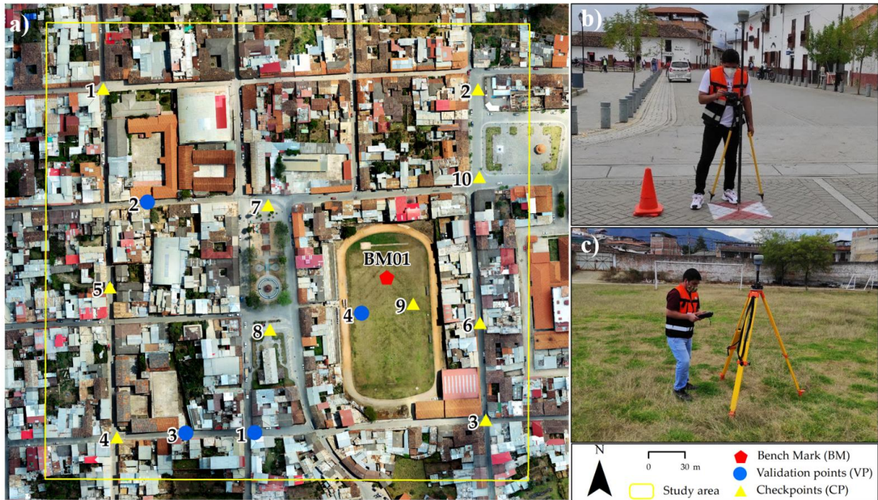
Figure 2. Photogrammetric Data Acquisition Process. (a) GCP distribution. (b) Target measurement. (c) Base station BM-01.
