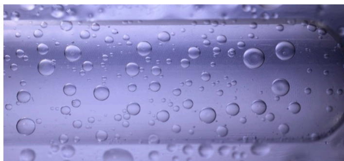
Figure 3. A photograph of the collected water droplets on the glass slide with silicone oil.
