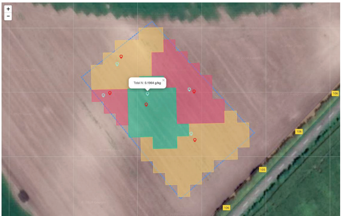
Figure 15. Fertilization prescription map generated based on the measurement results. Red pins represent proposed sampling locations by AI algorithm, while green pins represent actual sampling locations.
