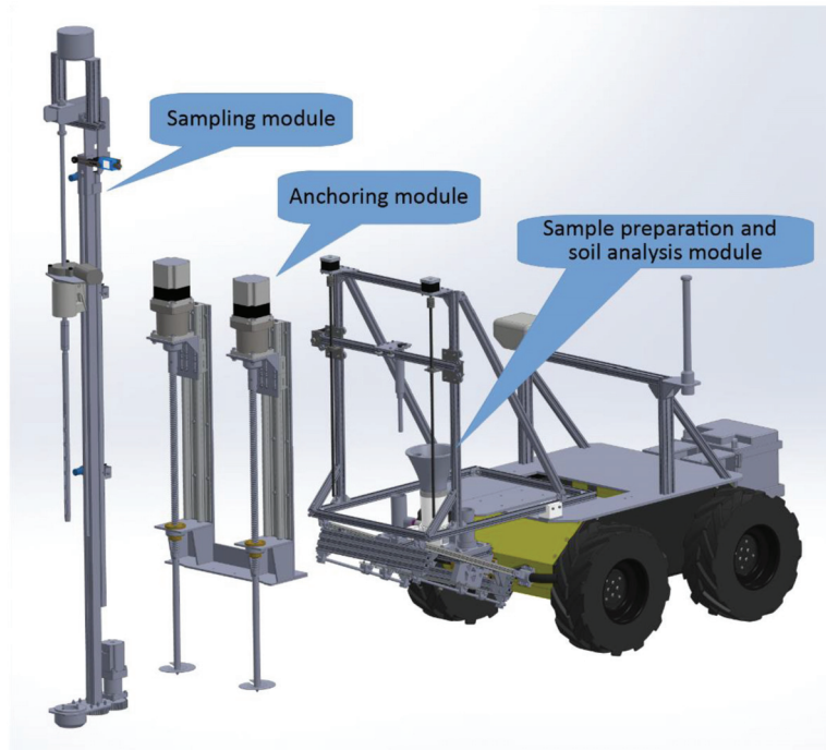
Figure 4. The 3D model of the exploded view of the agrobot Lala model.
