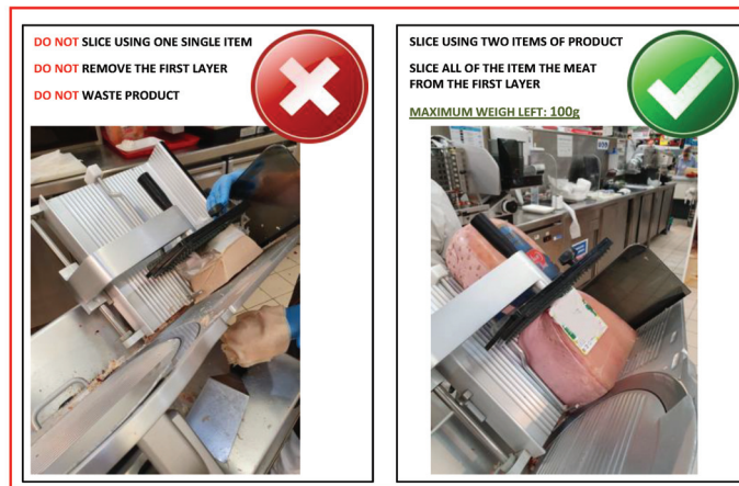
Figure 4. Visual standard for the “ham-cutting” operation created during the Kaizen event.
