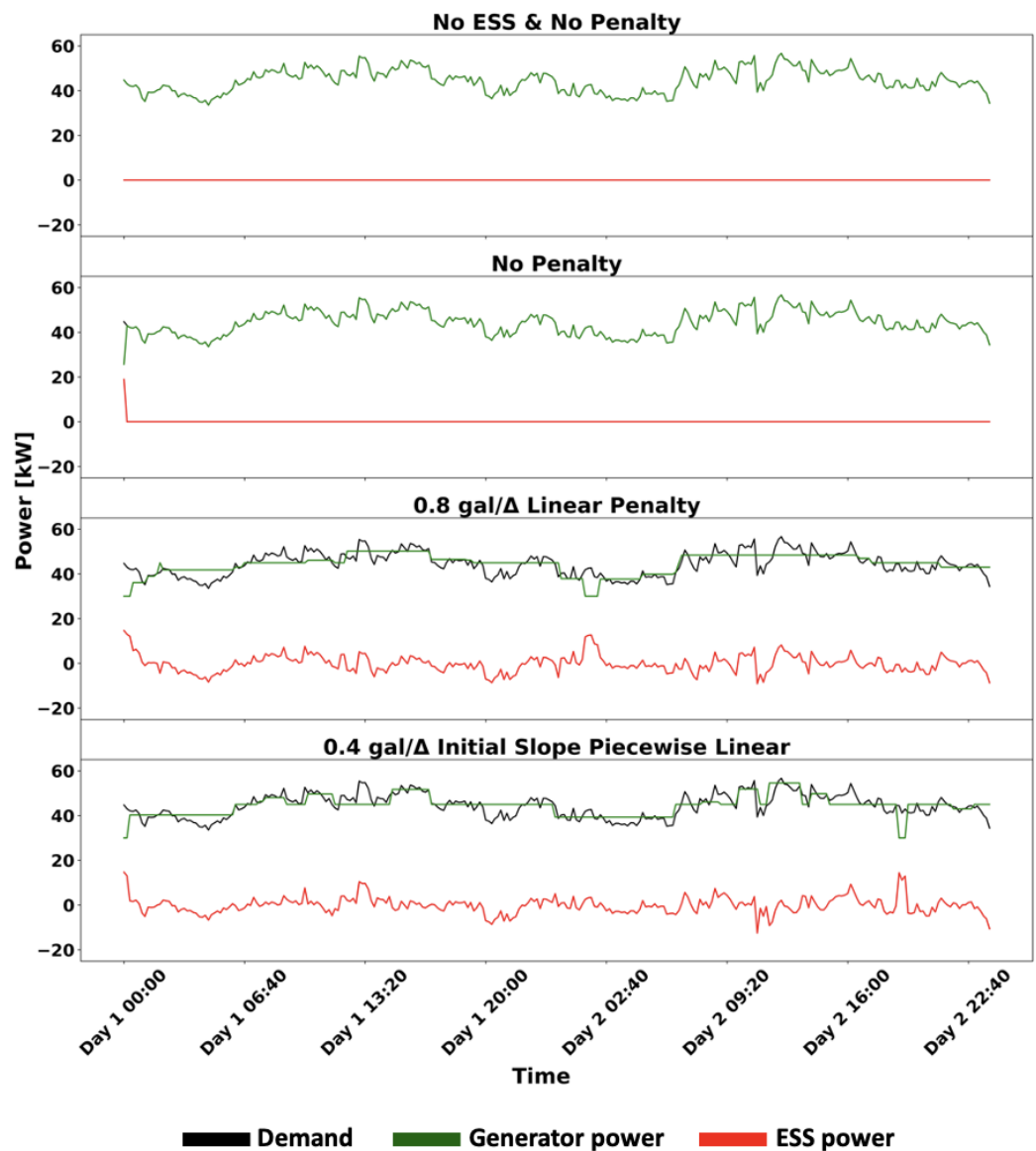
Figure 11. Optimal power distribution over various architectures for the summer demand scenario.
