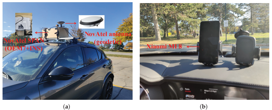
Figure 3. Photos of experimental setup. (a) experimental vehicle and setup, (b) experimental smartphones.
