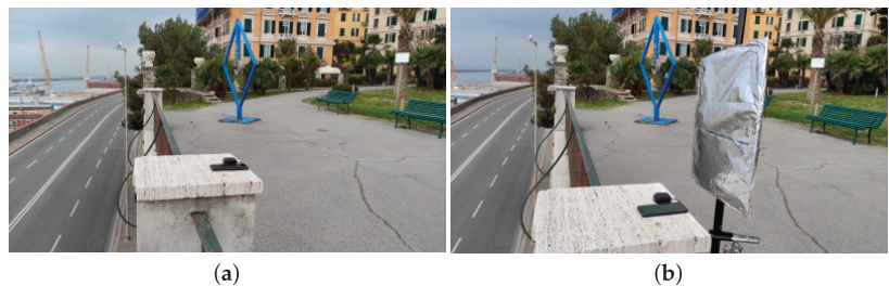
Figure 2. Test 2 acquisition under standard condition (a), and with multipath induced (b).
