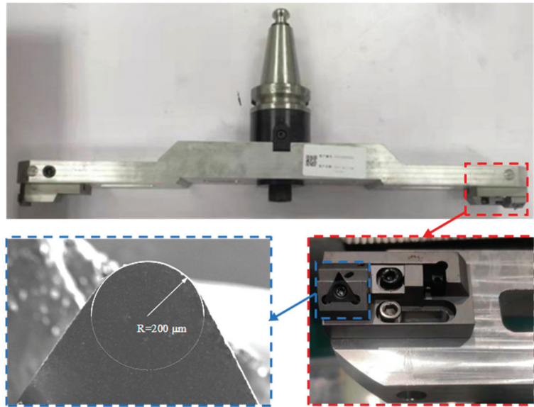
Figure 3. Specialized design cutting tool.
