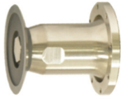
Figure 4. UCK (Ø63 mm Disc) cutting tool used in RUM experimental for HCs core workpiece.
