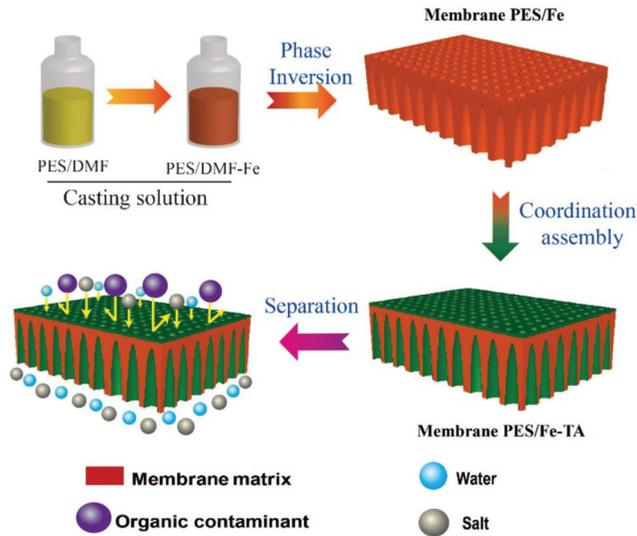
**Figure 2.** Schematic representation of the fabrication process of loss nanofiltration membrane and selective separation of dye and salt.
