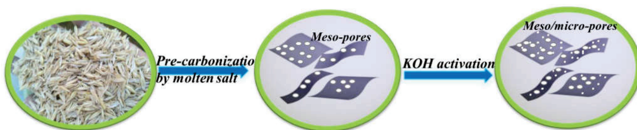
Scheme 1. Schematic synthesis process for the HPC.
