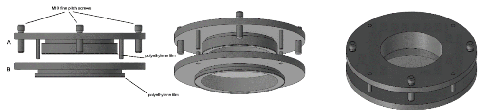
Figure 2. The figure shows a drawing of the device with the two membranes which seal the bottom of two containers A and B and the way it is assembled.
