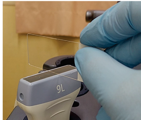
Figure 11. Simple educational materials that help provide an understanding of the influence of machine settings on the configuration of vertical artifacts. A glass microscope slide is placed perpendicularly on the footprint of a linear transducer with a thin layer of ultrasound gel.
