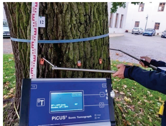
Figure 3. Stem geometry measurement with the electronic PiCUS Caliper (photo by M. Dudkiewicz, 2021).
