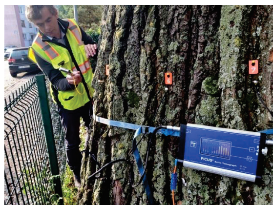
Figure 4. PiCUS sonic tomograph central unit and tree trunk measurement (photo by M. Dudkiewicz, 2021).
