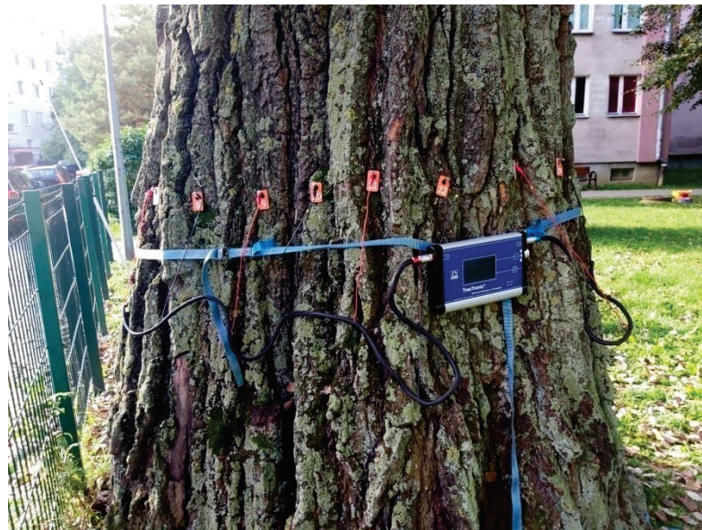
Figure 5. Tree measurement with the Picus TreeTronic electric tomograph (photo by M. Dudkiewicz, 2021).
