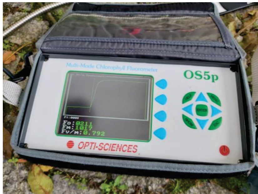
Figure 6. Advanced Fluorometer OS5p+ to measure the photosynthesis process (photo by M. Dudkiewicz, 2021).
