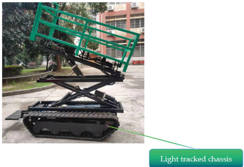
Figure 2. Electric fruit picking platform used for experimental trials.
