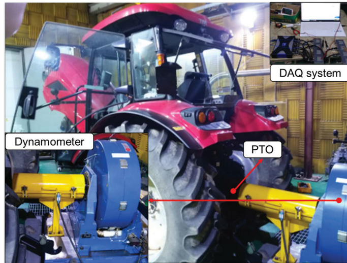
Figure 3. The PTO dynamometer test bench used in this study.
