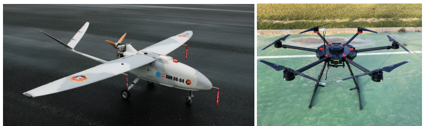
Figure 2. The Atlantic I (left) and DJI M600 (right) UAS will be used to validate the UTM functionalities developed in the GAUSS project.
