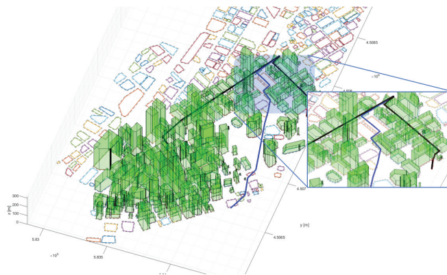
Figure 21. Example of a 3-D geofence wrapping a “turn” flight plan for sUAS_2 . The sUAS_2 trajectory is shown in black, and the sUAS_1 trajectory is shown in blue. Polyhedra (green) denote keep-out geofences around buildings. The remaining 2-D polygons denote keep-out geofences around buildings that are outside the combined ROI.
