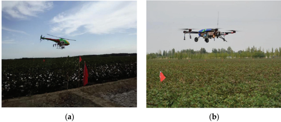
Figure 5. HY-B-15L single-rotor plant protection unmanned helicopter for cotton defoliant spray (a) and TXA616 plant protection UAV for rice growth regulator spray (b) [46].
