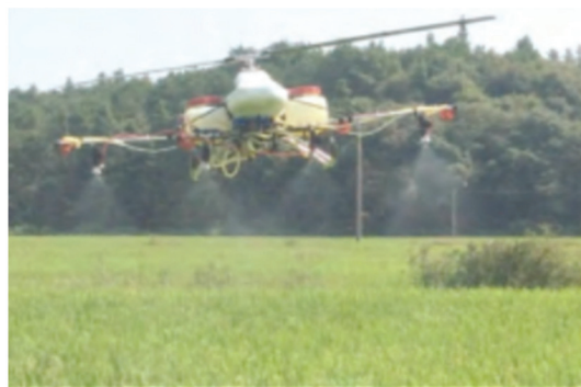
Figure 2. Rice field test with an XY8D UAV-based electrostatic spray system [31].
