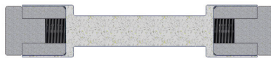
Figure 9. Cross section of the rotor, revealing the outer aluminium hull and the inner ferromagnetic cores.
