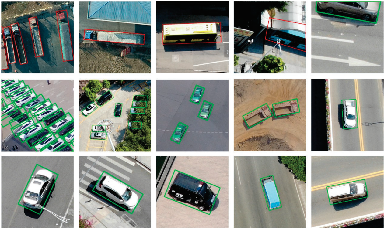
Figure 4. Samples of annotated images in VSAI (left to right, top to bottom). Large trucks belong to LV, a large truck (LV), a bus marked with an arbitrary quadrilateral bounding box (LV), a car labeled using an arbitrary quadrilateral bounding box (SV), cars densely arranged and mutually blocked (SV), cars partially occluded by vegetation (SV), a taxi (SV), small trucks (SV), pickup (SV), car (SV), SUV (SV), police car (SV), box truck (SV), minibus (SV).
