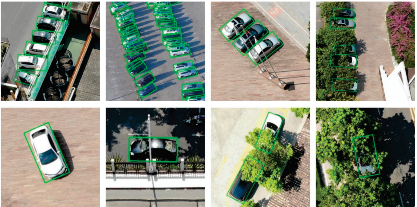
Figure 13. Examples of vehicle occlusion. The first line demonstrates different block reasons of instances, from left to right , occluded by a building, blocked by other vehicles, sheltered by shafts, such as flags, and occluded by vegetation, respectively. The second line illustrates different occlusion ratios, from left to right , no occlusion, small occlusion, moderate occlusion, and large occlusion.
