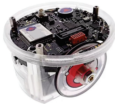
Figure 7. E-puck2 robot platform. E-puck2 is the latest mini mobile robot developed by GCtronic and EPFL, which is an evolution of the successful E-puck robot used in many research and educational institutes.
