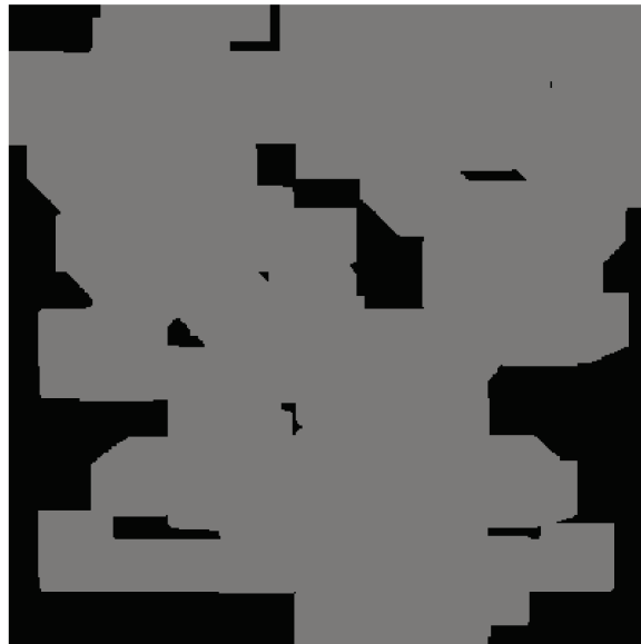
Figure 10. Coverage example with 10 agents, 78.02% coverage. The grey area depicts the coverage that the agents succeeded as a group in 180 s.
