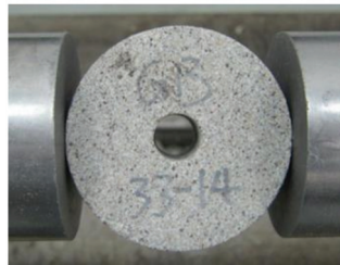
Figure 3. Clamping method of the specimen.
