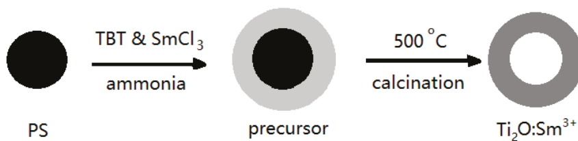
Figure 2. Schematic illustration of the formation mechanism for hollow TiO 2 :Sm 3+ spheres [29].
