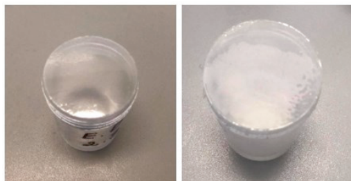
Figure 13. Water vapor transmission rate (WVTR) test. Films before (left) and after (right).
