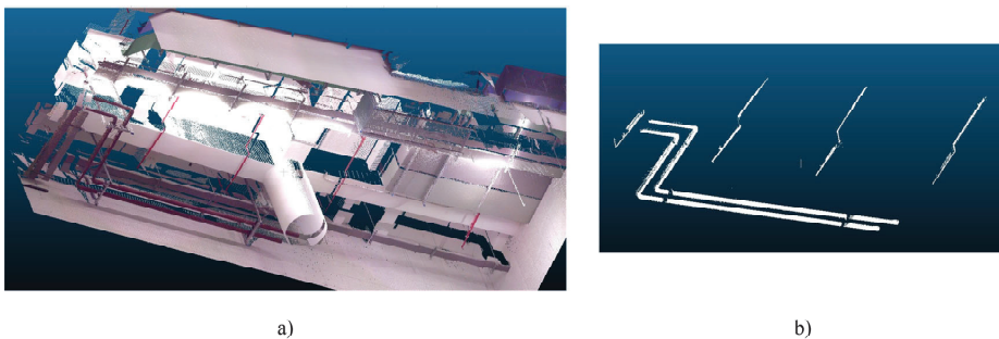
Figure 7. The point cloud dataset. (a) is the engineering scene dataset and (b) is showing extracted pipelines.
