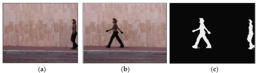
Figure 2. Pedestrian detection results in a single-frame image. (a) The initial frame, (b) the current frame, and (c) the detection result of ghost area.
