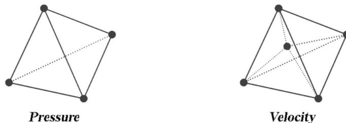
Figure 3. Degrees of freedom for the velocity and pressure for the tetrahedral element P1+/P1.
