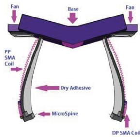
Figure 46. System composed of the SMA actuators, the structure and the cooling system for the soft gripper. Reprinted with permission from ref. [66]. Copyright 2021 IEEE.
