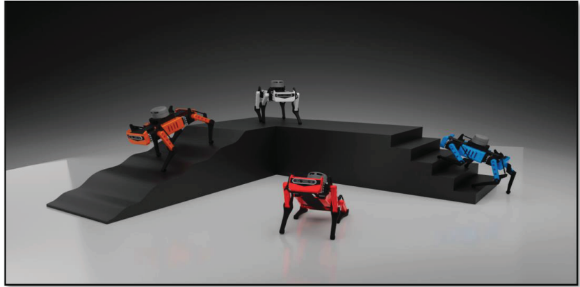
Figure 1. Iron Dog mini, a low-cost quadruped robot with Watt six-bar linkage mechanism.
