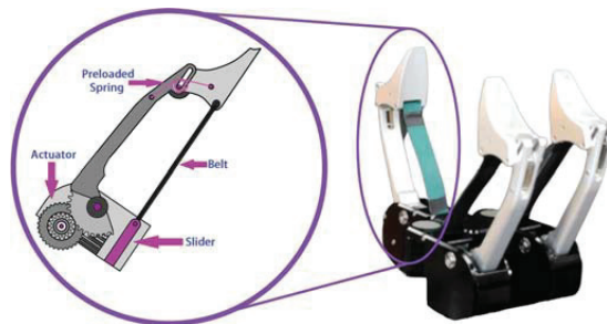
Figure 31. Double actuated gear and belt system of the gripper. Reprinted with permission from ref. [58]. Copyright 2020 IEEE.
