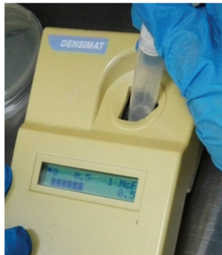
Figure 6. Measurement of the turbidity of the sodium microorganism suspension solution.
