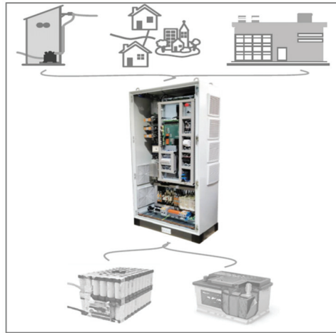
Figure 7. PED as developed in the project shows possibilities to integrate multiple batteries (at the bottom), as well as to use them in multiple contexts (on top).
