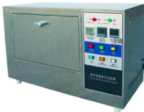
Figure 2. UV aging environment box for asphalt.
