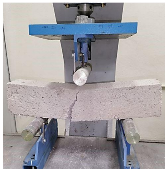
Figure 6. Apparatus for three-point bending test.
