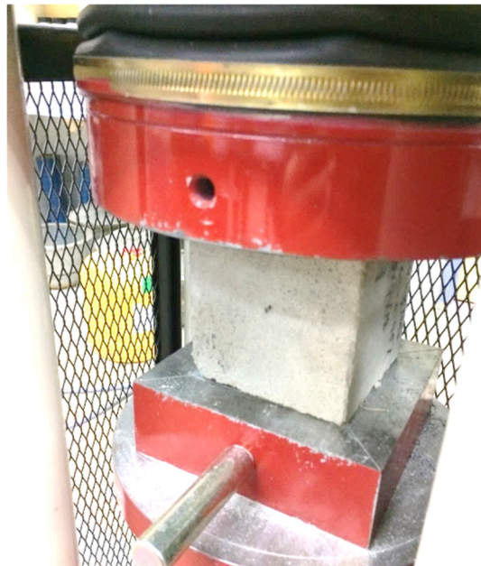
Figure 5. Setup for compression test.
