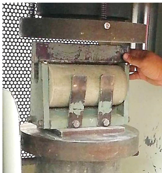
Figure 7. Splitting tensile test apparatus.
