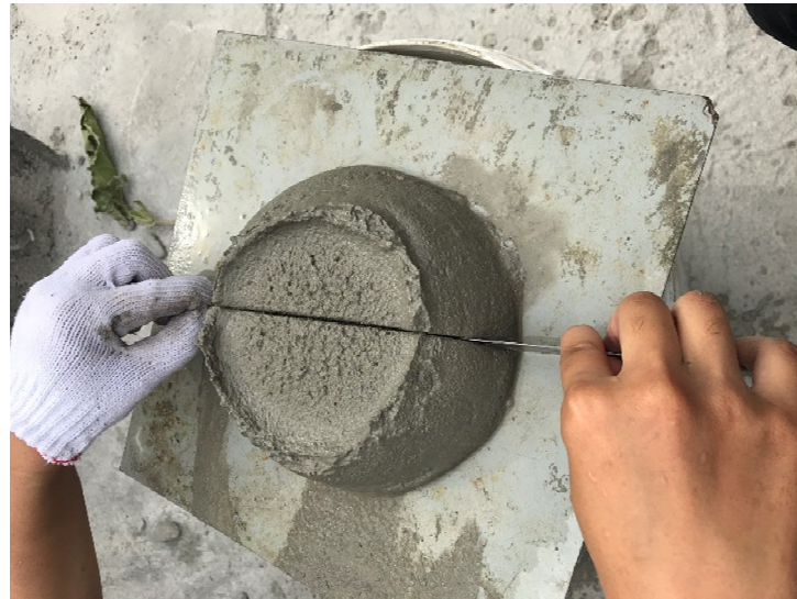
Figure 3. Measurement of the spreadability of foamed concrete.
