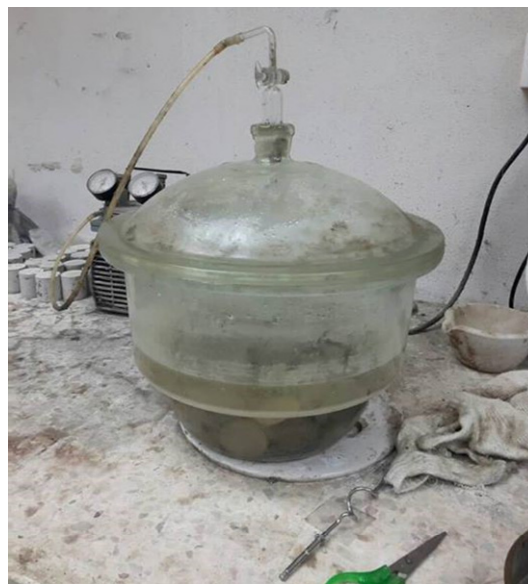
Figure 4. Vacuum saturation procedure.
