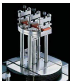
Figure 6. The clamp of Dynamic Mechanical Analysis.
