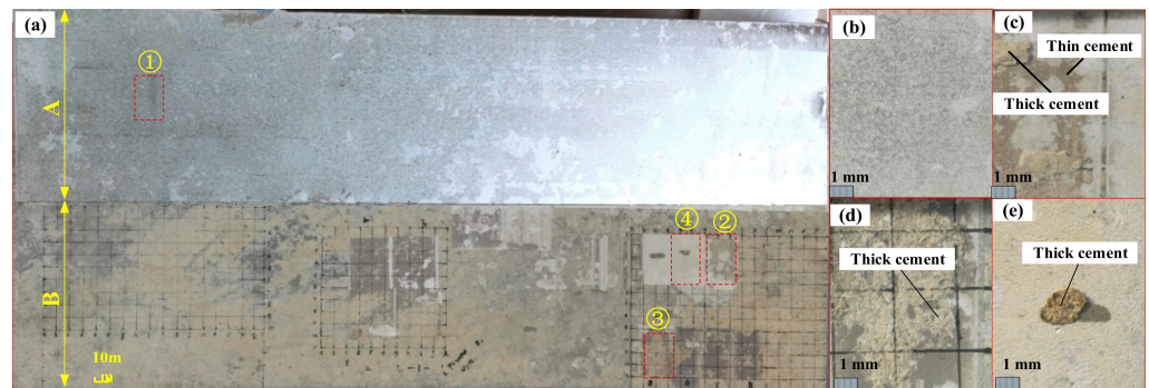
Figure 4. Macroscopic morphology and local magnification of cleaning surface: (a) Overall appearance of aluminum formwork; (b–e) ①~④ area enlargements.
