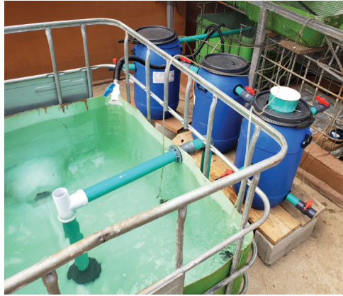
Figure 5. SANFU II RAS prototype implementation. Source: Authors.
