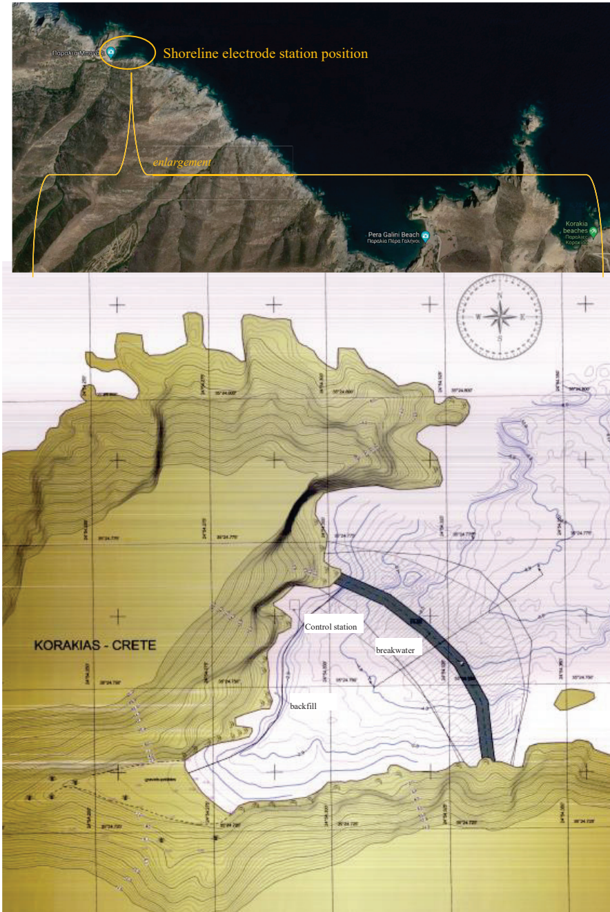
Figure 12. Shoreline electrode station at Korakia beach, Crete [78].
