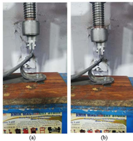
Figure 6. (a) Initial 0 mm displacement in the heel section; (b) 10 mm displacement under static load.
