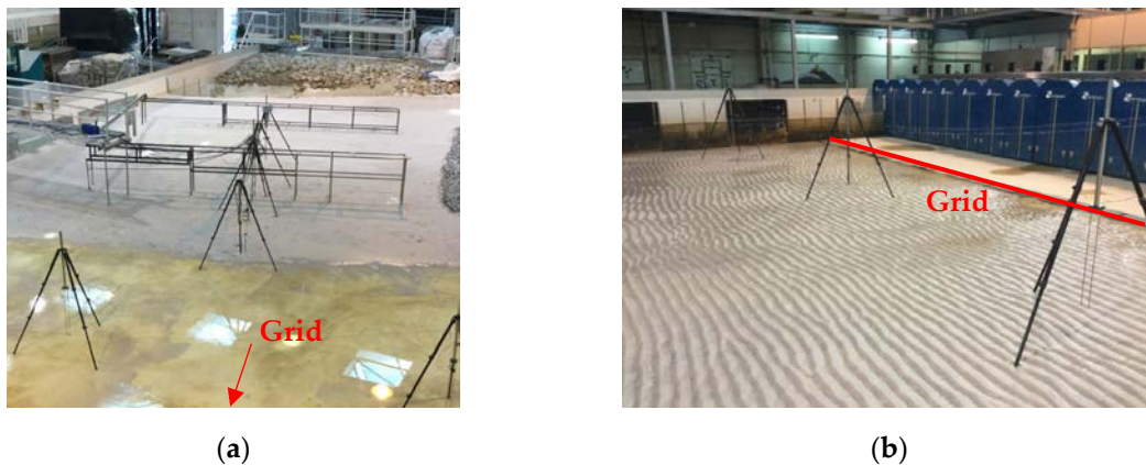
Figure 12. Offshore beach limits for scenario A: (a) Initial offshore profile limit (A.1); (b) Final offshore profile limit (A.1).
