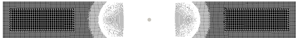
Figure 5. Example of a mesh generated by SnappyHexMesh , which was used for the simulative parameter studies of the influence of the particle shape on the overall pressure drop. To achieve reliable data, the refinement differs depending on the relative location of the particle and the channel walls. In this case, the film thickness between the particle and the channel was 0.
