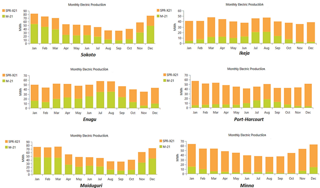
Figure 7. Monthly electricity generated by the PV/WT/battery-based charging station in the six selected sites.
