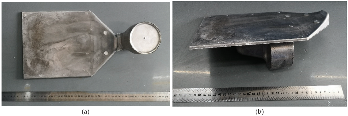
Figure 10. AlSn20Cu alloy billet produced using semi-solid die casting: (a) front view, and (b) side view.
