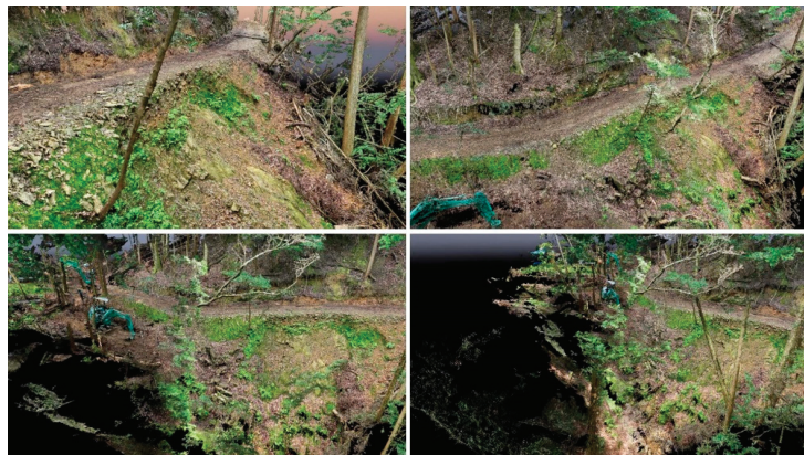
Figure 1. A 3D model generated by SfM analysis before the repair work started.
