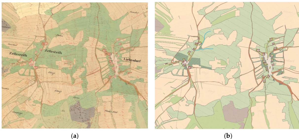
Figure 2. Imperial Obligatory Imprints of the Stable Cadastre 1:2880 : (a) example of a georeferenced scan of a map sheet used for vectorisation; (b) vectorisation of the map sheet shown in (a).
