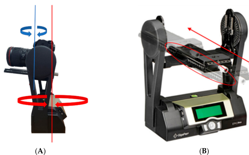
Figure 3. Panoramic instrument of GigaPan EPIC Pro V. (A) Eccentric issue caused by different axes of rotation between panoramic instrument (red part) and camera (blue part); (B) Adjustable position (scale marks) to put camera (red part).
