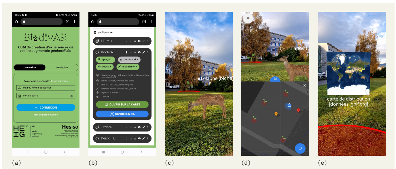
Figure 10. BiodivAR 's mobile user interface: (a) login; (b) all available bioverses sorted by categories (authored by user, public, bookmarked); (c) AR view after opening a bioverse; (d) a collapsible 2D map for navigation; (e) view of a media showing the distribution map of an adjacent specimen's species, after entering a POI's radius.
