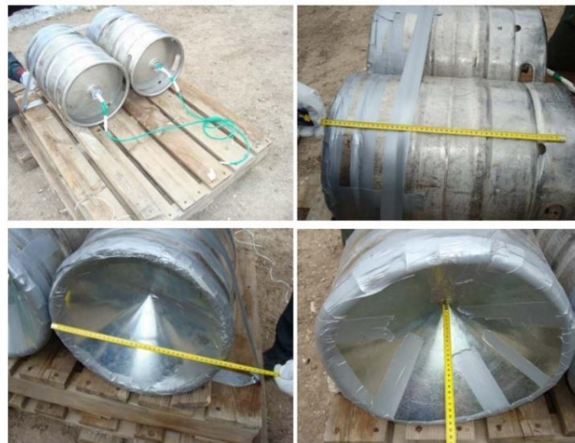
Figure 1. Directed charges of 42 kg of TNT.
