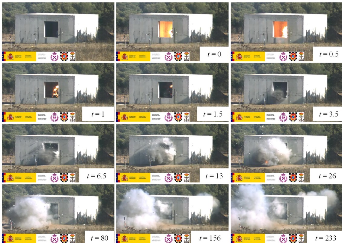
Figure 5. Sequence of images obtained with HSC in trial T4: ANFO. Time in milliseconds; the reference time is the first frame of the video where the detonation is observed.
