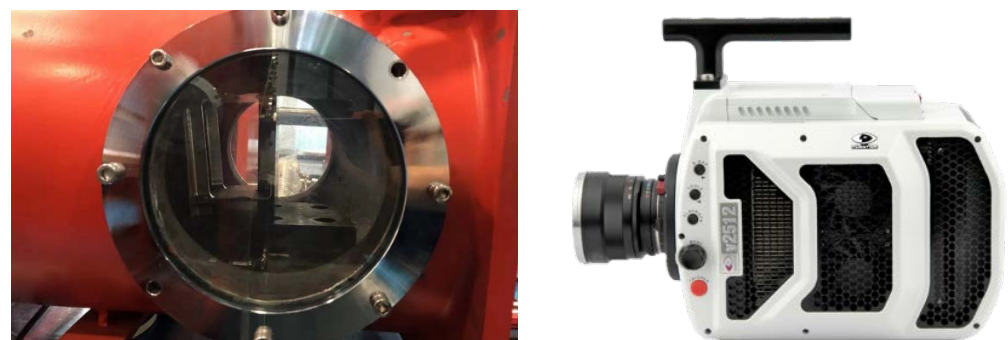
Figure 4. Observation section setting of the target chamber.
