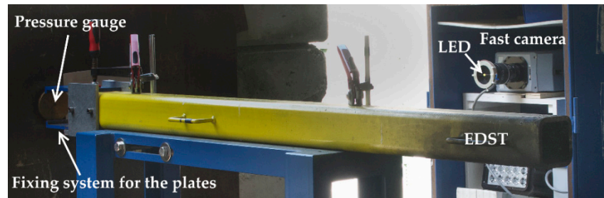
Figure 3. View of the experimental setup, showing the explosive driven shock tube and the high speed camera with the LED.
