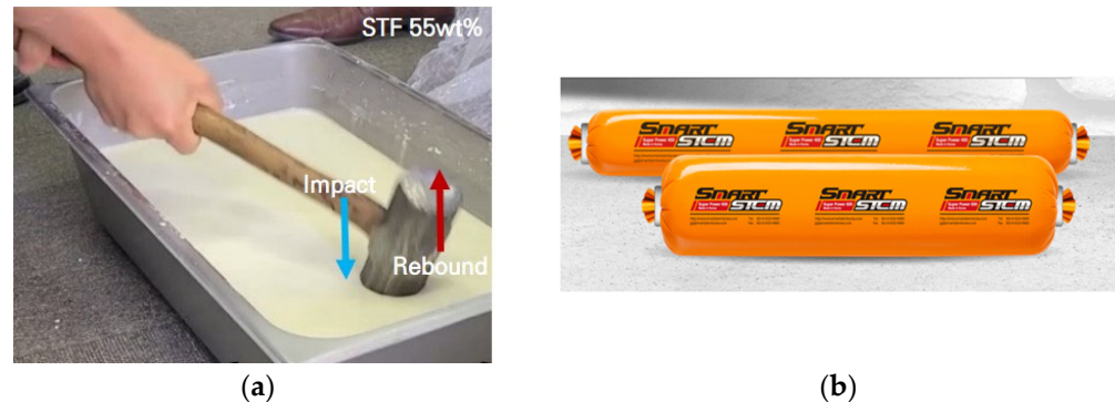
Figure 4. (a) Shear thickening fluid-based stemming material image and (b) package products.
