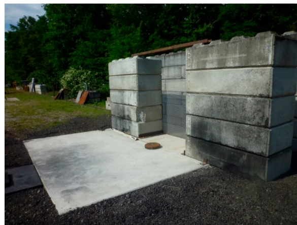
Figure 6. View of the experimental setup showing the one-grid configuration: the grid position, concrete blocks and gauge in front of the grid.
