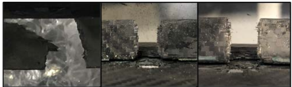
Figure 10. Typical damage mode of composite stringer.
