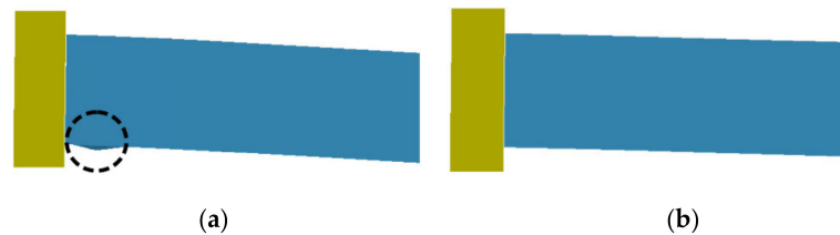
Figure 19. Failure mode of CFDST column with: (a) normal strength concrete and (b) UHPC [21]. Copyright permission obtained from authors.
