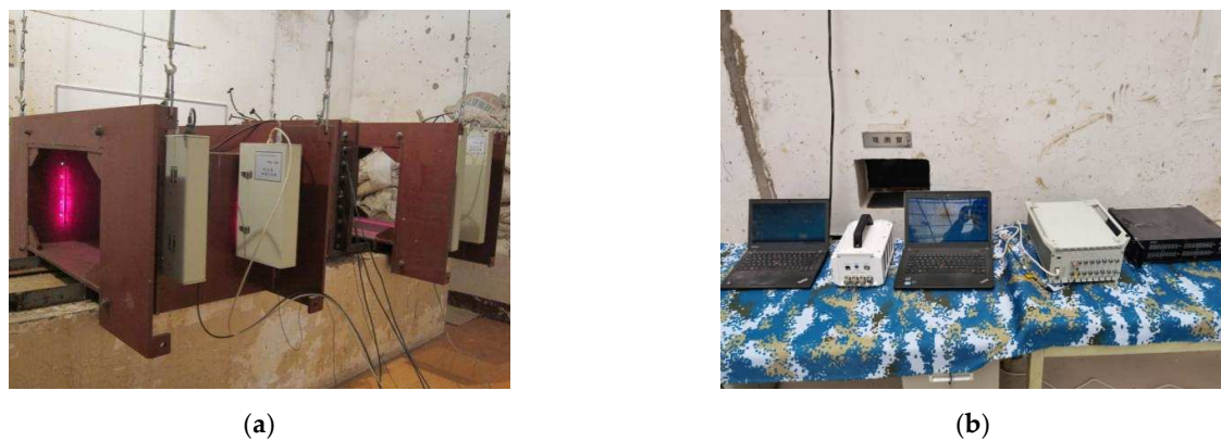
Figure 2. Test equipment and recording devices. (a) Laser velocimeter; (b) high-speed camera, pressure sensor and target-net velocimeter.
