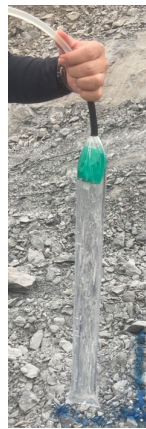
(c) Water tube for hydraulic pressure measurement
