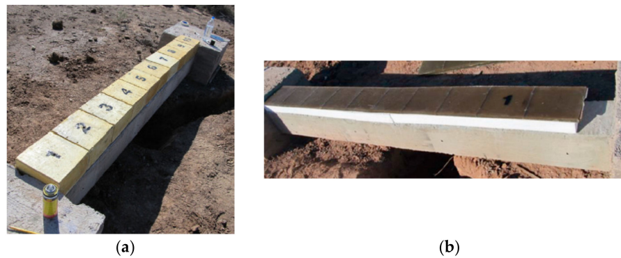
Figure 12. RC columns reinforced with: (a) polyurethane bricks [15,16] and (b) resin panels and insulation layer [22]. Copyright permission obtained from authors.
