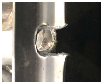
Figure 18. Top skin damage in Situation 3.
