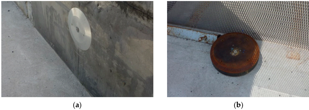
Figure 7. (a) Reflected pressure gauge located on the wall behind the grids; (b) pressure gauge located in front of the first grid position.
