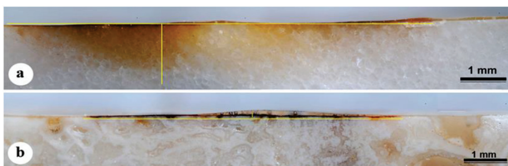
Figure 3. Artificially stained samples. Cross sections images acquired in reflected light (10 \times ) of Carrara marble (a) and Travertine (b) stained outdoors for two seasons (spring and summer).
