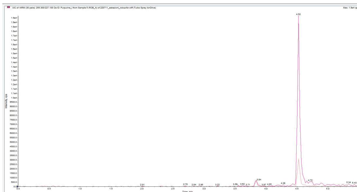
Figure 8. Purpurin chromatogram relative to agar gel (3% w/v ) madder extraction from wool. The darker chromatogram refers to the transition from 255 to 227 m/z , while the lighter chromatogram refers to the transition from 255 to 171 m/z .
