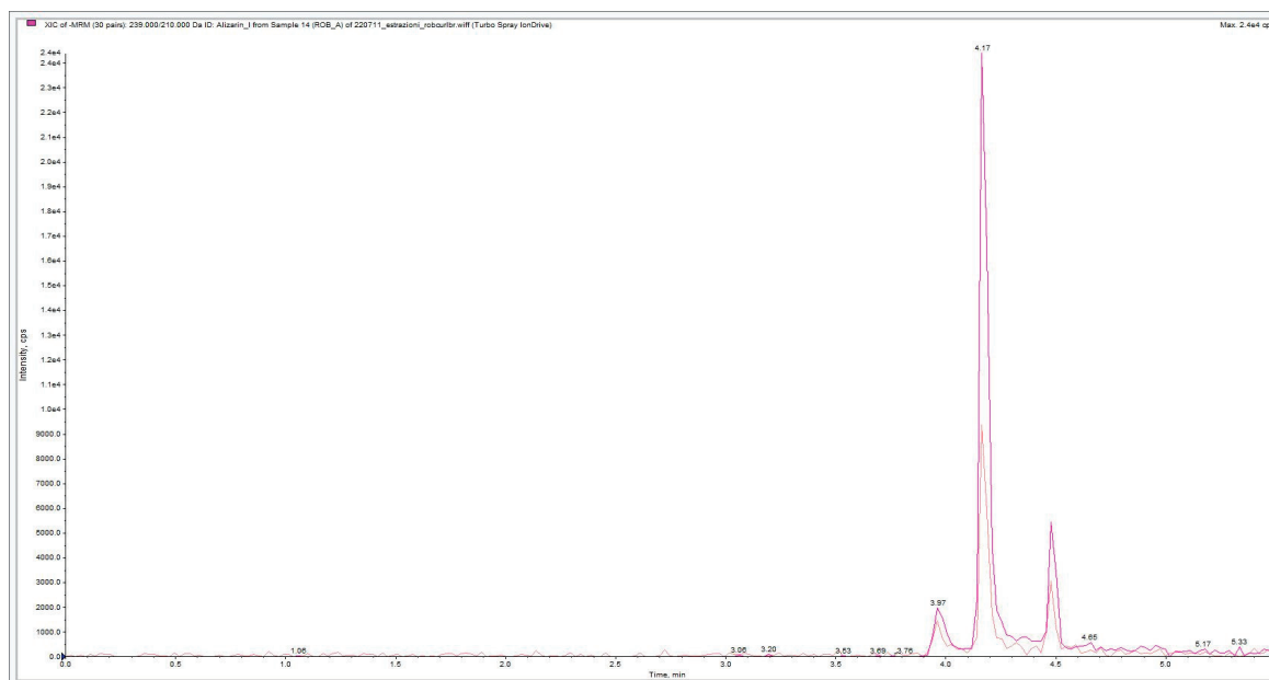
Figure 7. Alizarin chromatogram relative to agar gel (3% w/v ) madder extraction from wool. The chromatogram in darker pink refers to the transition from 239 to 210 m/z , while the chromatogram in lighter pink refers to the transition from 239 to 167 m/z .
