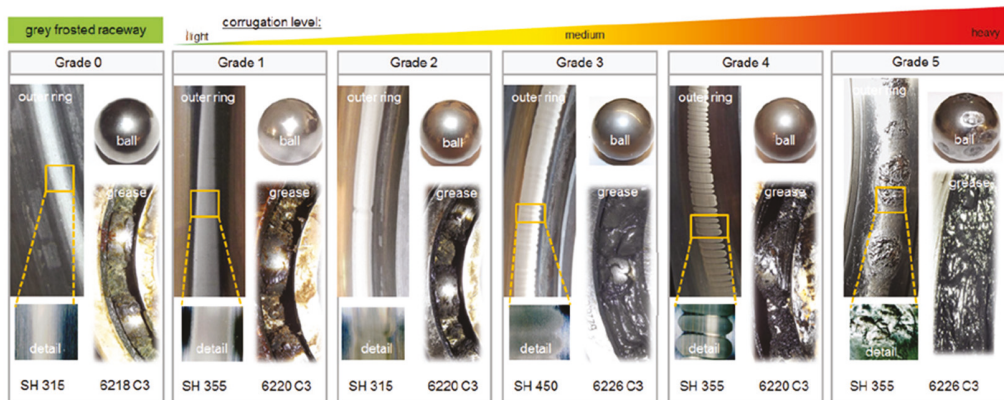
Figure 1. Different grades of bearing damages. ©2018 IEEE. Reprinted, with permission, from [17].
