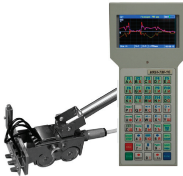
Figure 5. Tester of Stress Concentration TSC-4M-16 and scanning 4-channel sensor.
