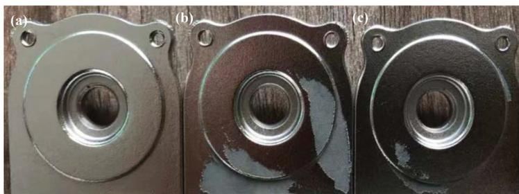
**Figure 11.** Digital macrographs of PEI samples: (a) standard condition (4 min), (b) short acceleration time (2 min), (c) excessive acceleration time (10 min).
