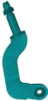
Figure 9. Boom finite element model.
