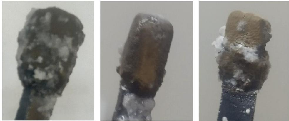
**Figure 2.** Photographs of the cathode deposits obtained after the electrolysis of the  $\text{KCl-K}_2\text{SiF}_6$  melt at a temperature of  $790\text{ }^\circ\text{C}$  and cathode overvoltage of 0.25, 0.15, and 0.1 V vs. QRE potential.
