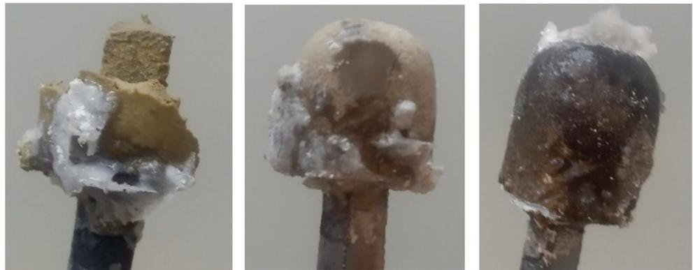
**Figure 3.** Photographs of the cathode deposits obtained after the electrolysis of the  $\text{KCl-K}_2\text{SiF}_6\text{-SiO}_2$  melt at a temperature of  $790\text{ }^\circ\text{C}$  and cathode overvoltage of 0.25, 0.15, and 0.1 V vs. QRE potential.
